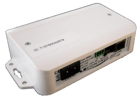
LS SmartConnect Gateway is a device for connecting controllers with ModBus to the Internet (IoT). Our software ensures a secure connection to the internet without having to configure the router.
